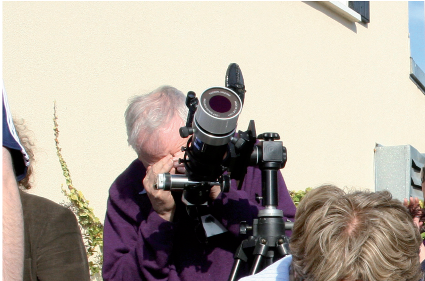
Observing the Sun using a custom fitting glass solar filter at the objective. Often, a telescope user would remove the finderscope to prevent inadvertent stray light and heat from the Sun to cause damage. Photo by the author.
